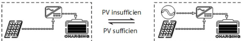
4) Only Solar (Only Solar): Only PV charging, without Mains charging. This is the most energy-efficient way in which battery is charged only by solar panels, and is usually used in areas with good lighting conditions.
