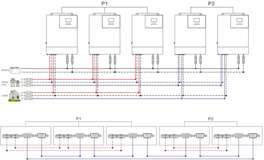
e) **Six all-in-one solar charge inverters of the system connected in two phase:**
