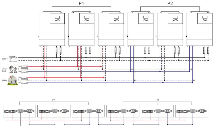
**Parallel Operation in three phase (for U and S series model):**
