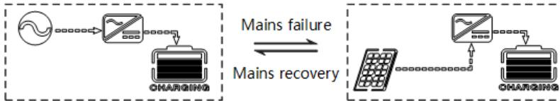
3) Hybrid charging: PV and mains hybrid charging. PV MPPT charging is a priority, and when PV energy is insufficient, the mains supply supplements. When the PV energy is sufficient again, the mains stops charging. This is the fastest charging mode, suitable for the areas where power grid is unstable, providing sufficient backup power supply at any time.
