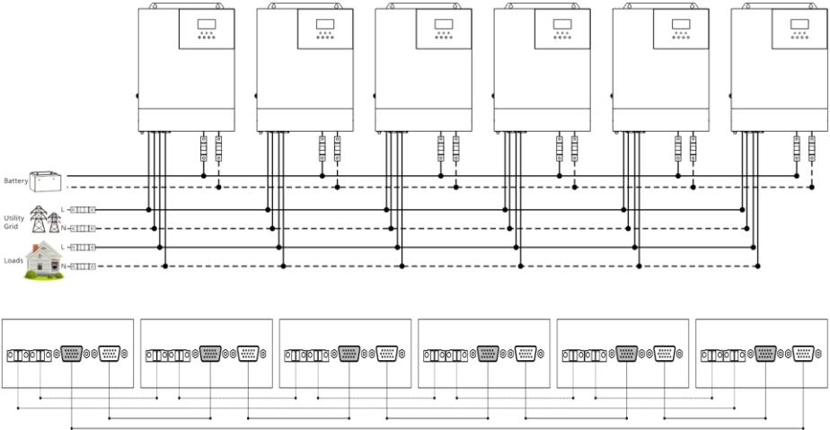
**2.4.4 Schematic diagram of parallel connection in split phase**
