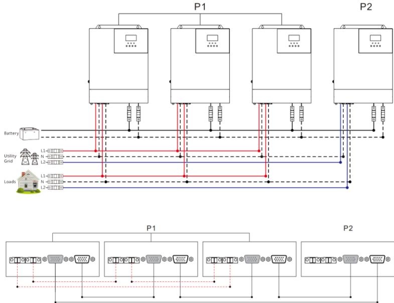
**d) Five all-in-one solar charger inverters of the system connected in two phase:**
