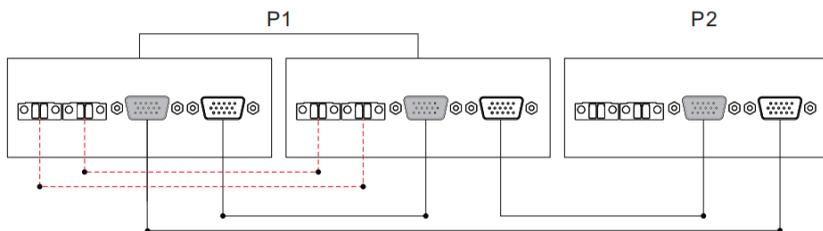
c) **Four all-in-one solar charge inverters of the system connected in two phase:
